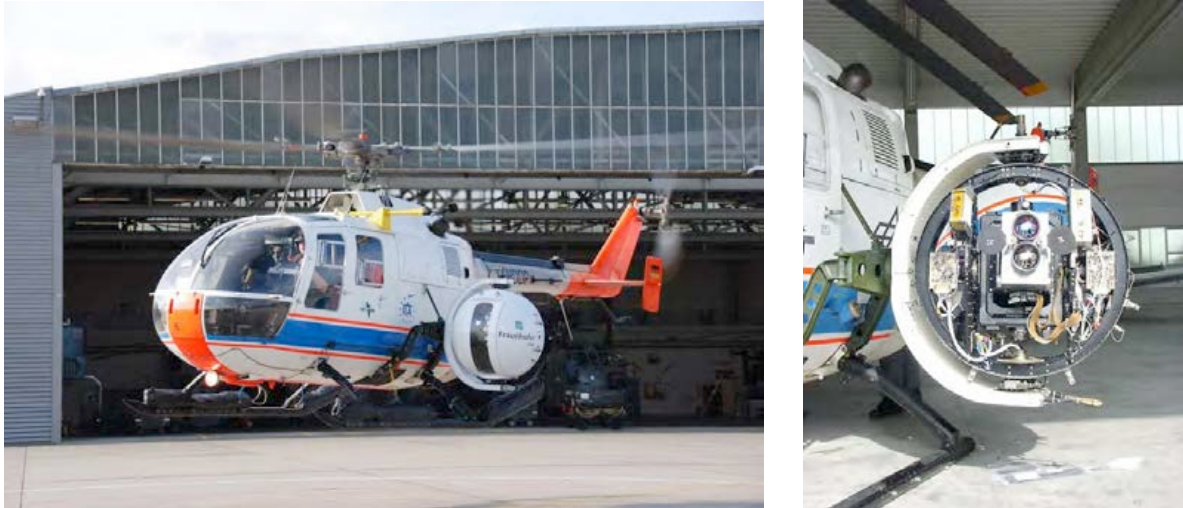
Figure 0-9: AIR-Sig system mounted on the helicopter BO-105 (left) and AIR-Sig sensor (right)
